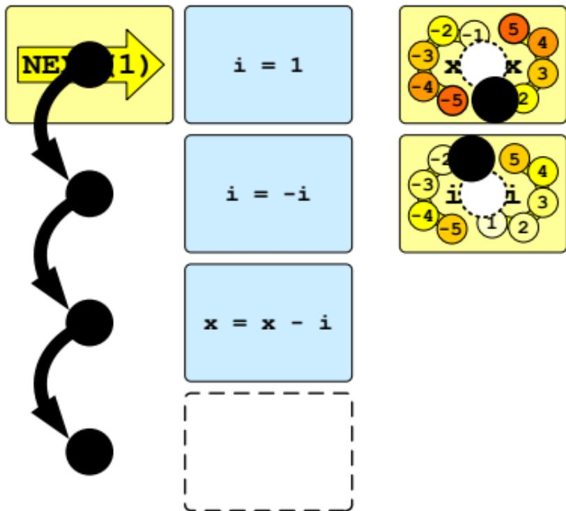
In this example, advancing the **NEXT** pointer consists of executing the instruction to which it points, and then sliding it down to the next card. Advancing it three times
